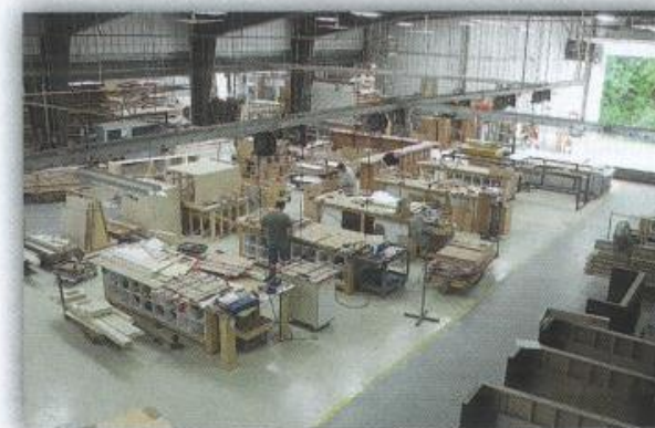
The custom production cell includes the bench work area where skilled craftsmen make custom projects.
