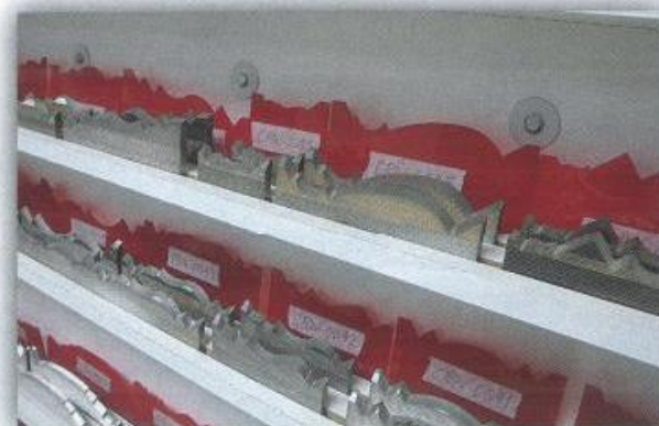
Tooling profiles are stored in an easy-to-see display in the tool room. Mouldings are produced and finished here.
