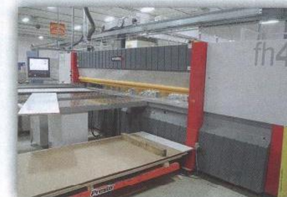
Schelling fh4 panel saw was recently added, along with an automated panel retrieval system.
