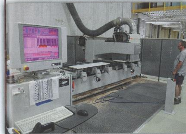
The casework production area has a Holz-Her Pro-Master point-to-point machine.
