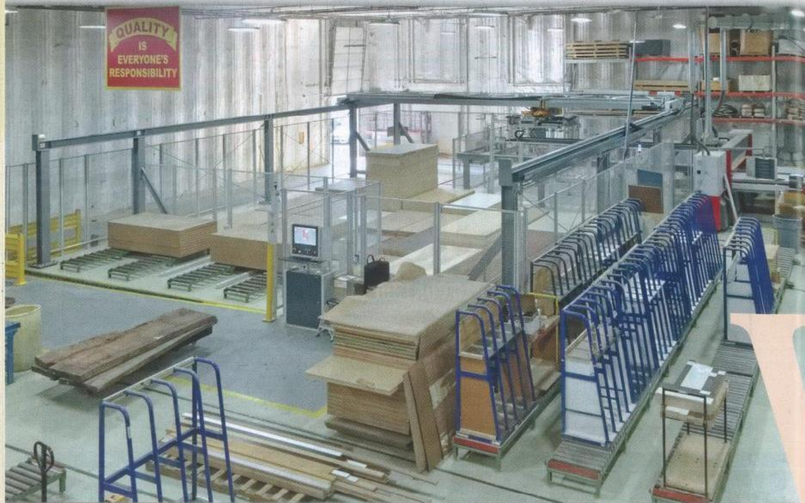
The AmeriCase production area is separate and includes the new Schelling fh4 saw and VS 12 storage and retrieval system.
